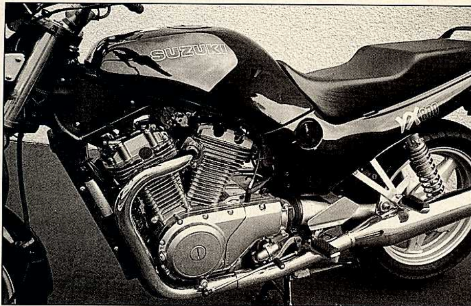
The slim-line design of the fuel tank belies its 5.0-gallon capacity, which gives the VX800 a cruising range of well over 200 miles on a fillup.
