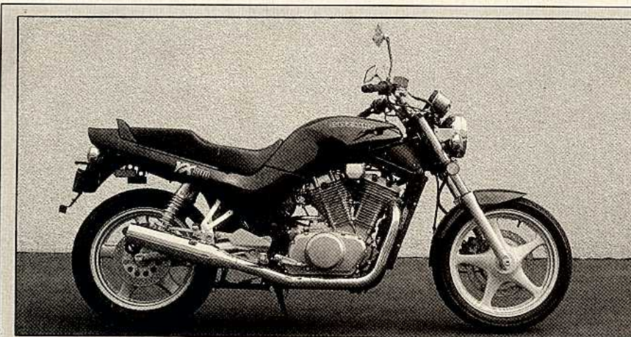
The slim-line design of the fuel tank belies its 5.0-gallon capacity, which gives the VX800 a cruising range of well over 200 miles on a fillup.
